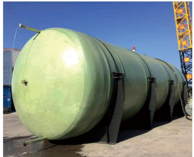
试水 water testing
