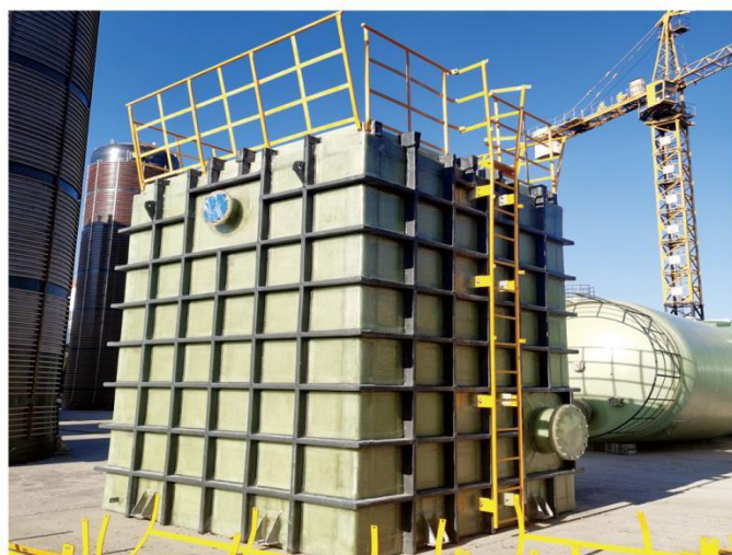
盐酸洗涤槽 Hydrochloric acid washing tank
